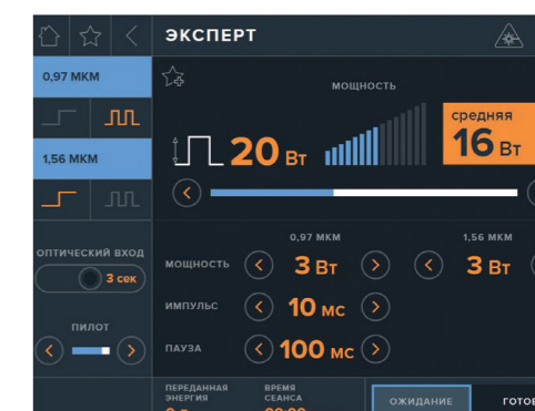
In "Expert" mode FiberLase S allows for controlling two independent radiations (0,97 and 1,55 μm) through one fiber instrument
