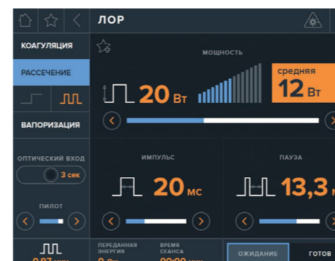
In the "ENT" mode the wavelength of the laser radiation is set automatically when the soft tissue exposure mode is selected
