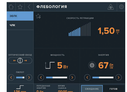
In "Phlebology" mode, the energy is automatically calculated based on the selected power and retraction rate parameters
