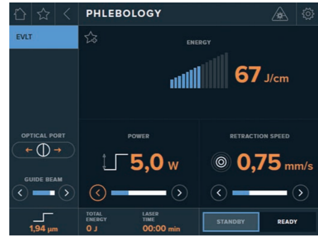
«PHLEBOLOGY» MODE The user is offered a recommended fiber extraction speed depending on laser parameters which are used.
