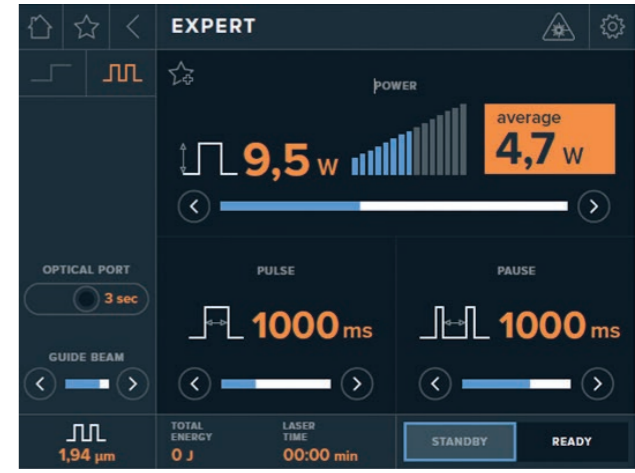
«EXPERT» MODE The user can choose continuous or pulse mode of operation, set the parameters of power, pulse duration and pause.
