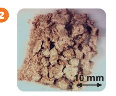
The special **«Ultra» pulse** fragmentation mode instantly breaks down the densest stones into large fragments for subsequent lithoextraction.
