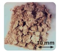
The special **«Ultra» pulse** fragmentation mode instantly breaks down the densest stones into large fragments for subsequent lithoexcavation.
